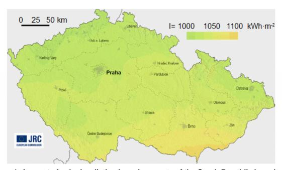
Figure 1. Amount of solar irradiation in various parts of the Czech Republic based on (ŠÚRI, 2010)
