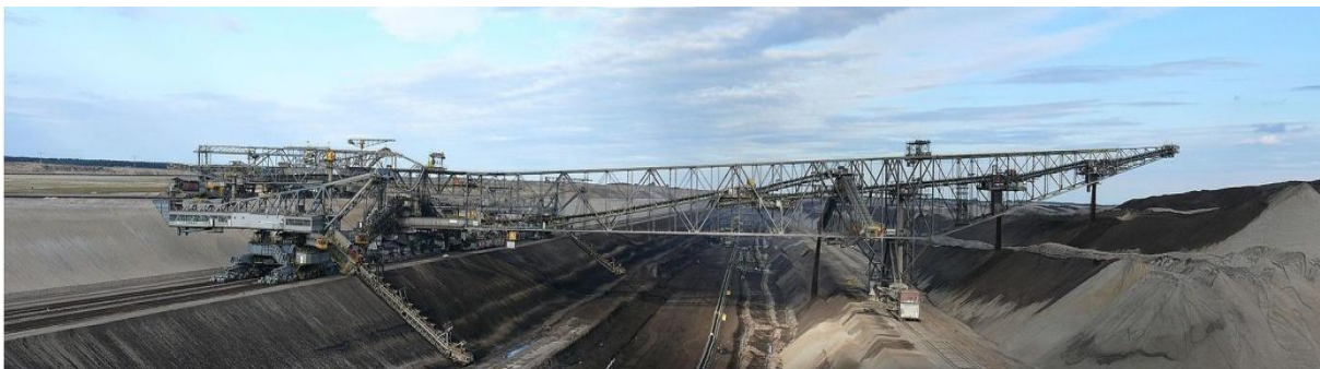
Figure 2: Overburden Conveyor Bridge - F60 in the 90' (source: Wikipedia, the free encyclopedia)
