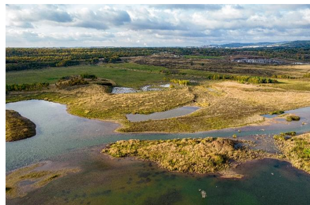
Figure 5 and 6 Breakdown of the originally straight bank of the Marcela reservoir on the internal spoil heap of the ČSA mine photo: Markéta Hendrychová
